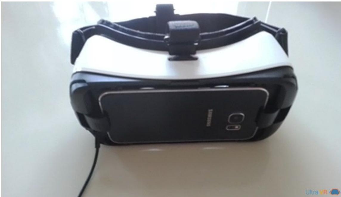
Navigation: The Touchpad, located at the right side of the Gear VR, is used for both selection and navigation of displayed elements.
